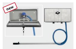
M22 M : M22 M. Injector ST-160 with metering valve ST-162. including chemical suction set comprising of suction hose DN 8 blue. 1.500 mm. suction filter ST-31. and chemical-resistant plastic tube. 320 mm. Max. 350 bar / 90° C
