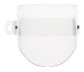
Clear Polycarbonate visor with 7 nylon strips layered together. The tabs on the strips pop-up one at a time for easy removal. Can be adjusted vertically for correct viewing height. This fully assembled T-N-Wear provides excellent clarity (perfect for painting) and gives excellent heat, chemical and scratch resistance.
