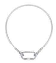
The AZ 410 connecting lanyard is a component of fall protection equipment. When combined with an energy absorber (e.g. ABM) it forms a connecting and shock absorbing device. The connecting lanyard is a portable anchor point complying with EN 795/B. The line is suitable for securing 3 users at a time using the AE 320 device. Steel cable fitted with loops with thimbles at both endings. The middle part of the lanyard is protected by a transparent plastic tube.
