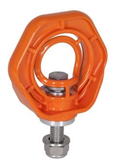
The anchor point AT185 is an anchor device according to EN 795 type A and serves to protect three people at the same time. The AT 185 anchorage point may only be used as personal protective equipment against falls from a height and cannot be used to lift loads. The device is made of AISI304 stainless steel casting and an aluminium sleeve on which the device can be freely rotated.
